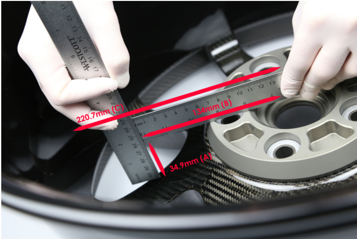
The A dimension is 34.9mm The B dimension is 134mm The C dimension is 220.7mm
